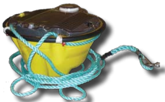
NOAA satellite buoy used for tracking marine debris such as ghost drift nets
